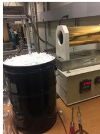
Insulation placed on the copper rod after heating
