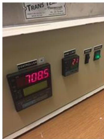
3.5 hours to reach 708 C with the tip of copper receiver at 1100 C
