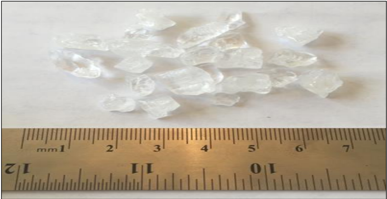
Figure: 1. Flux grown crystals of mixed alkali halide compounds doped with metallic impurities.
