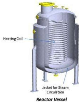
Fig. 2C - Cross Sections of the Reactor Vessel
