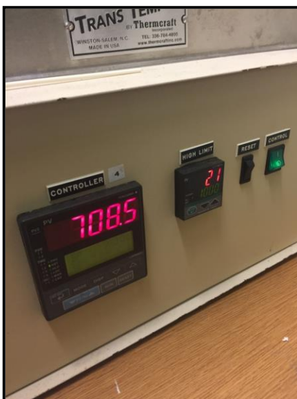
3.5 hours to reach 708 C with the tip of copper receiver at 1100 C at RPI, USA
