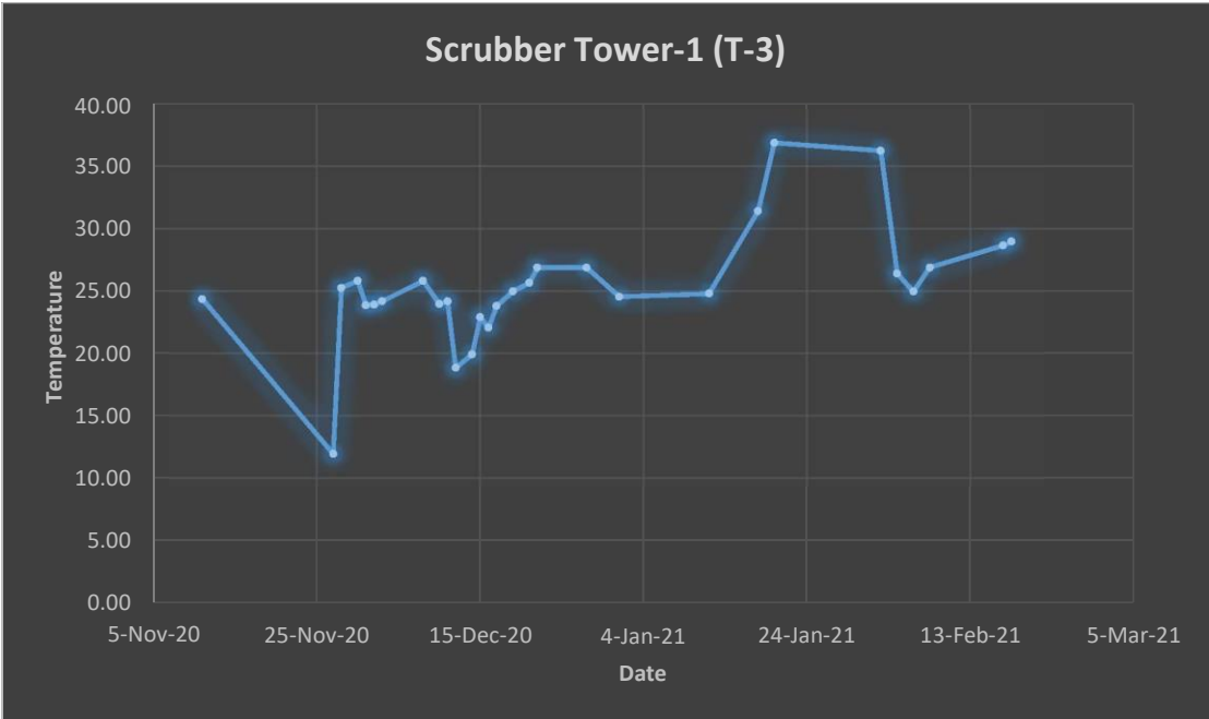
Graph 3: one Month Trial run result of temperature of water in Scrubber Tower-1
