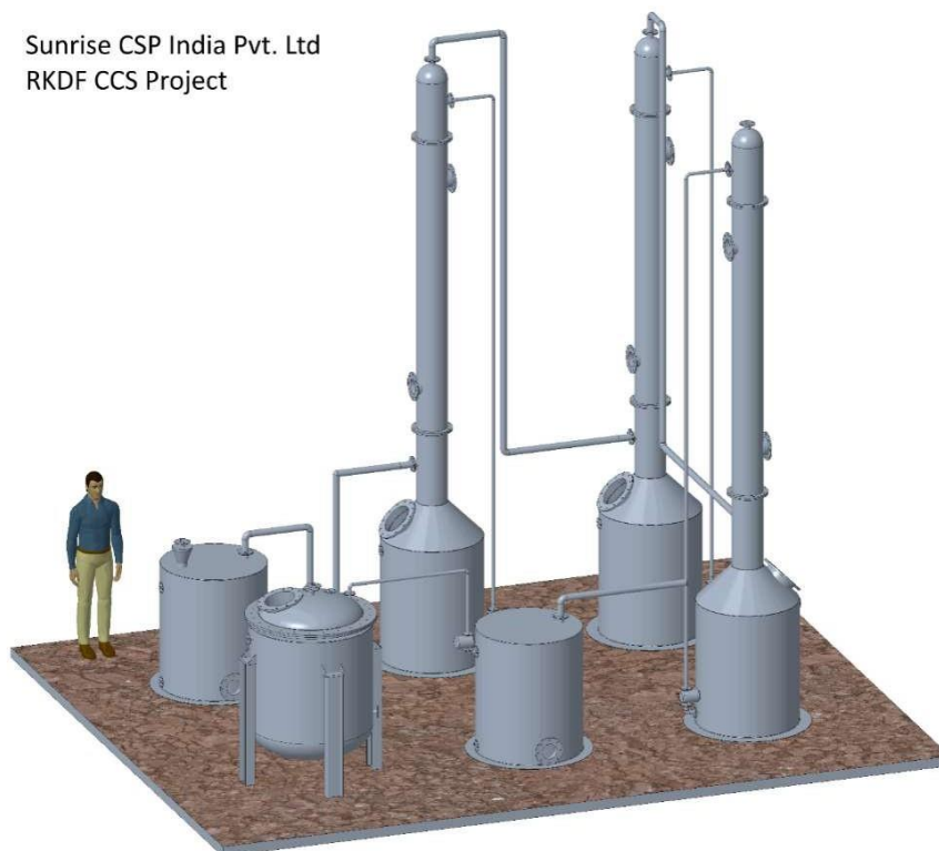
Figure 6: Depicts the setup for the CCS plant.
